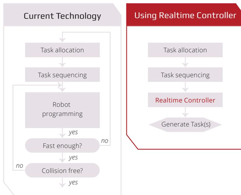
**The Realtime Controller was developed to eliminate the main bottleneck in multi-robot workcells.**
